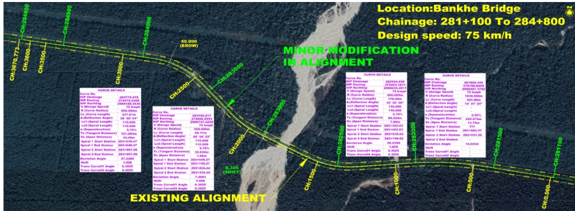
Figure 6-5: Alignment at Approaches of Bankhe Bridge
