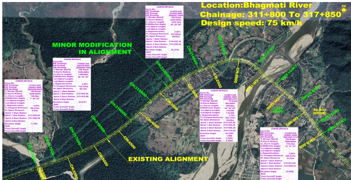
Figure 6-3: Alignment along Bagmati River Bridge and Approaches
