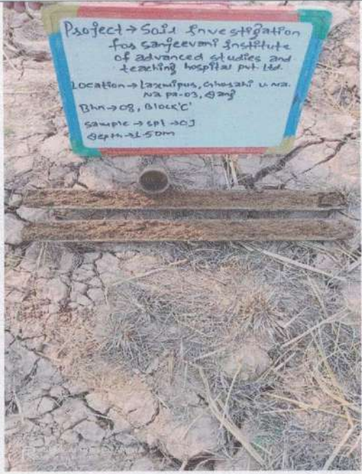
2. Drilling sample in BH8
