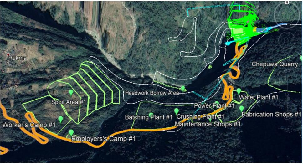
Figure 6.1: Headworks Area Proposed Ancillary Facilities
