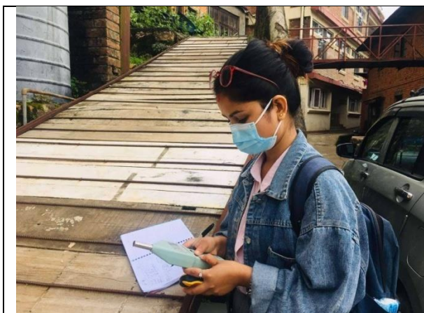
Plate 5-1: Measuring sound level using noise level meter
